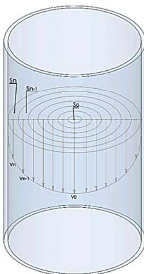
**Fig.18.** Velocity distribution in pipe flow
