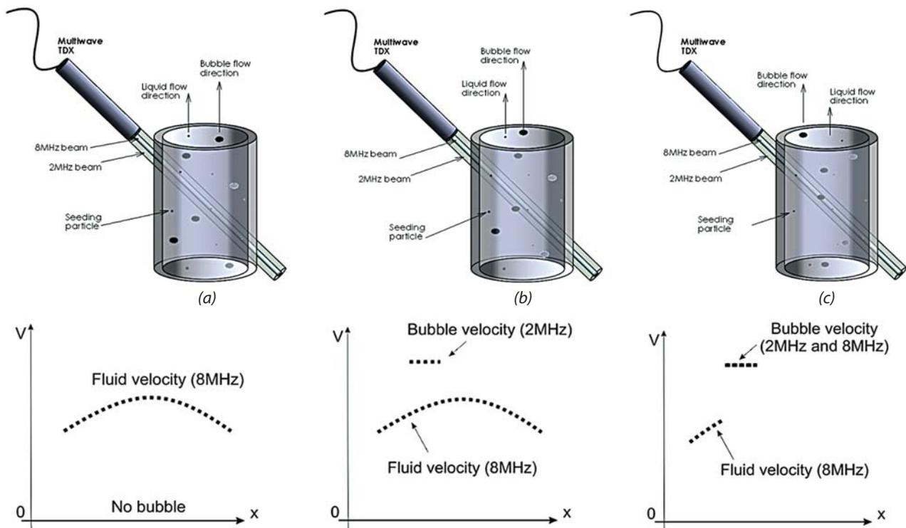
Fig.7. Relative positions of a bubble and ultrasound beams (up) and corresponding selection algorithms of valid liquid velocity (down)
