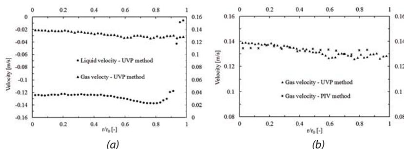
Fig.17. Measurement of two-phase flow: (a) liquid and gas velocity profile measured by UVP method; (b) gas velocity profile measured by UVP and PIV methods
