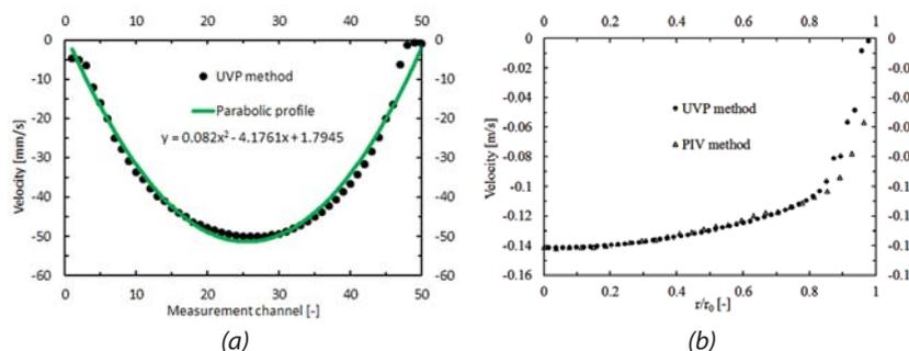
Fig.13. Measurement of single-phase flow: (a) fully developed laminar flow (Re=1400); (b) fully developed turbulent flow (Re = 8100)
