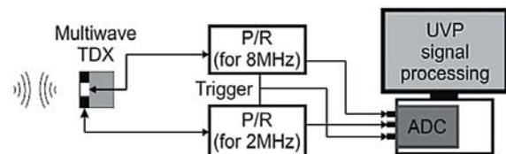
**Fig.10.** Schematic configuration of the multi-wave UVP system for measurement of single-phase and two-phase flows
