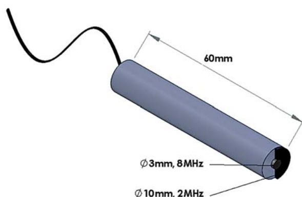
Fig.6. A schematic configuration of multi-wave ultrasonic TDX
