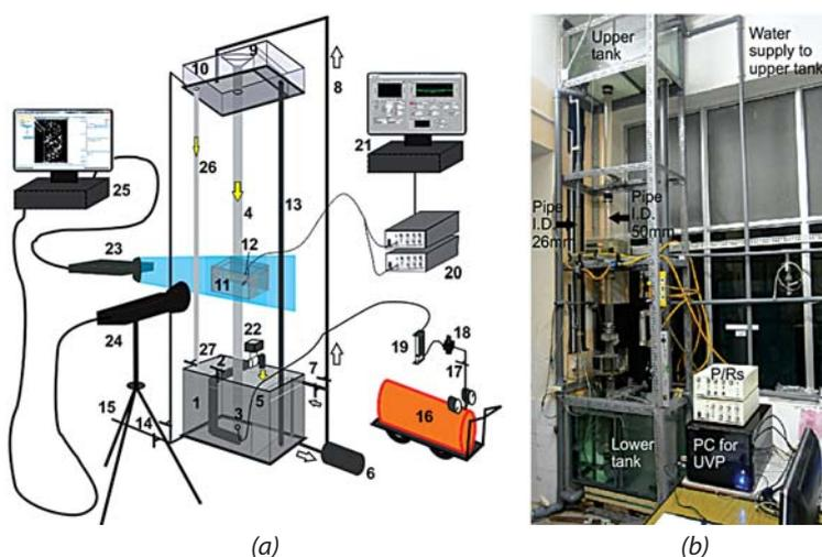
**Fig.8.** Schematic diagram of the experimental apparatus
