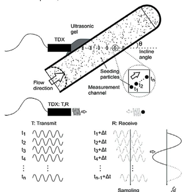
**Fig.1.** Principle of the Doppler method
