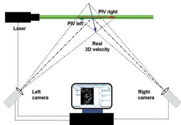
**Fig.11.** Schematic diagram of the Dantec 3D-PIV
