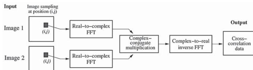
Fig.5. Schematic diagram of the algorithm of the displacement estimation based on Fourier transform (figure from [9])
