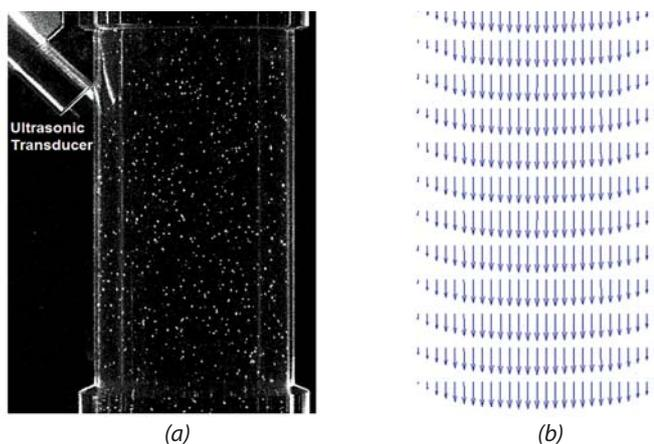
Fig.14. A typical particle image of single-phase flow (a) and 2D velocity field calculated by PIV method (b)
