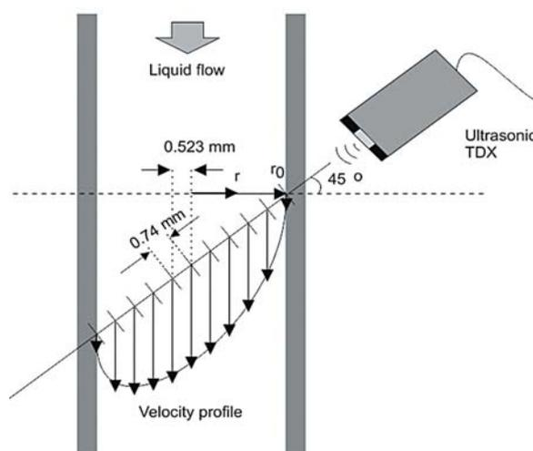
**Fig.12.** Arrangement of the ultrasonic TDX and pipe flow under measurement
