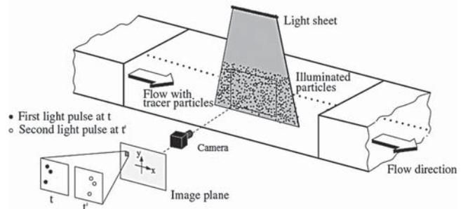
Fig.2. Schematic diagram of the PIV method [9]
