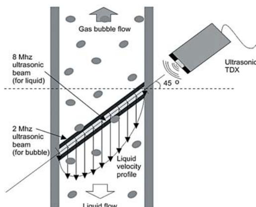
Fig.15. Arrangement of the multi-wave TDX and the two-phase flow in the pipe
