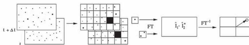
Fig.4. Schematic diagram of the displacement estimation method using Fourier transform [9]
