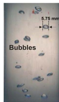
Fig.16. A typical bubble image by high speed camera
