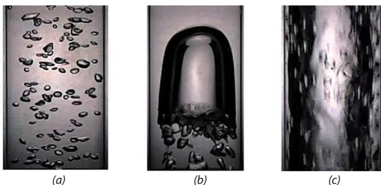
**Fig.9.** Typical two-phase flow regimes observed in the flow loop with 50mm I.D. pipe using a high speed camera (JVC Hybrid Camera GC-PX1, JVC Co. Ltd.) with frame rate 300Hz (a: bubbly flow; b: slug flow; c: annular flow)
