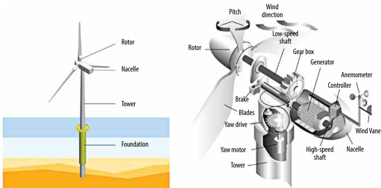
Figure 2. Configuration of the wind turbine technology assembly [4].
