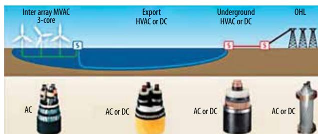
Figure 5. Types of offshore wind power cables [7].
