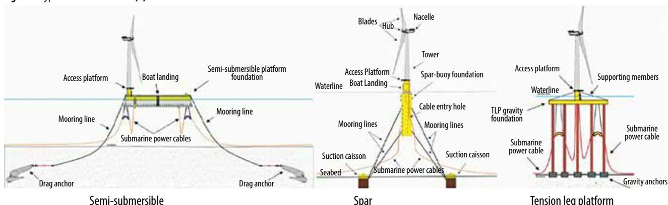
Figure 4. Types of floating foundations [6].
