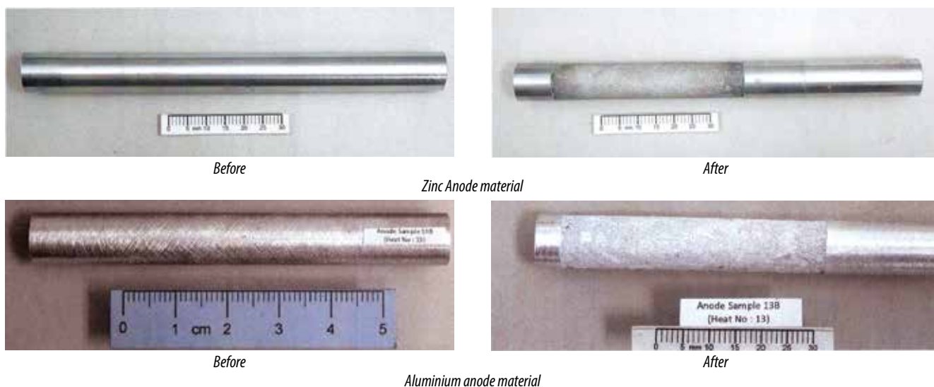
Figure 4. Images of sample surface before and after the electrochemical test.
